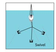
the nylon line, the surging waves and intense gusts are much more likely to yank the anchor out of the bottom. More and larger anchors (suited for the type of bottom) increase a boat's chances of staying put. Even more staying power can be had using the tandem anchoring technique – backing each anchor with a second anchor.
